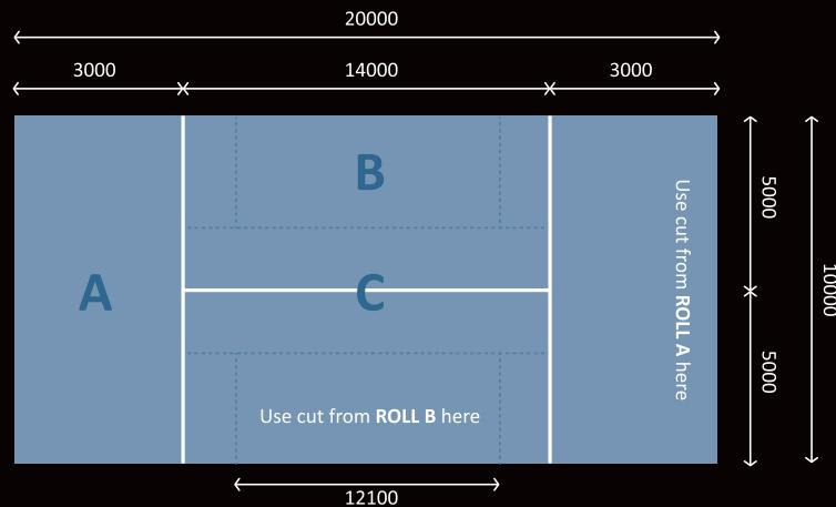
**ROLL A** Roll a (20m x 4m): to be split in half on site to create 2 rolls of 10m x 4m for both top & bottom base lines
