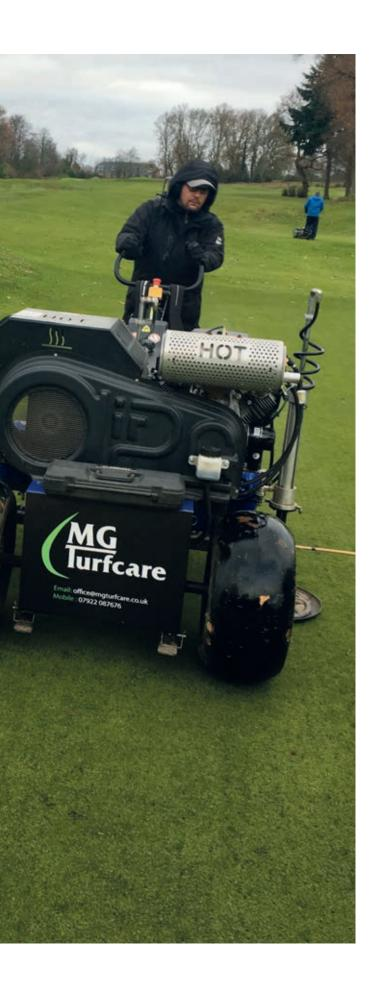
This allows greenkeepers to remove material, such as poor quality soil and thatch and allows water and air into the root zone.
