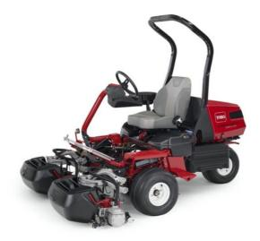
**Image caption:** Toro's ground-breaking first all-electric riding greensmower, the Greensmaster eTriFlex 3370 will be at BTME.
